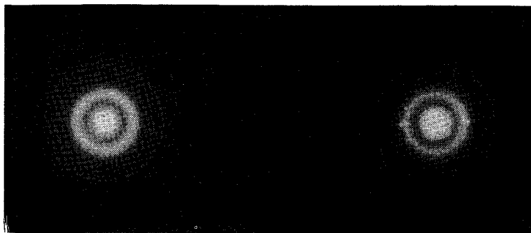
Fig. 13: X-Ray Spectra of Relaxed and Stretched Polybutadiene Cured with Standard Recipe Containing Zinc Oxide.
